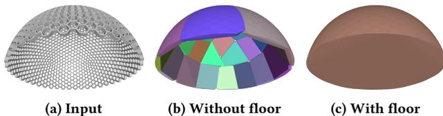
**Figure 5:** (a) A dome of small, tiled hexagons. (b) An automatic decomposition finds the interior navigable from below, and models it with 27 parts. (c) Using Eq. (5) to add a solid floor allows a single-part decomposition.
