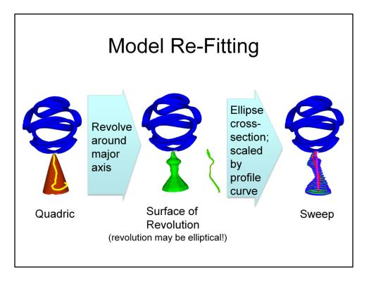
While we can of course interactively re-fit models from scratch, our system can also transform one type of fit directly into another.
