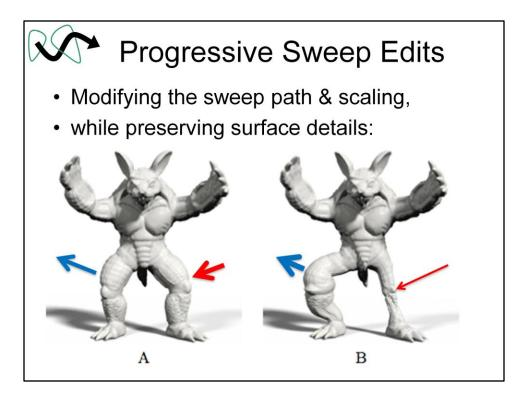
Here we edited the armadillo's legs by fitting sweeps to each leg, and then changing the sweep path and scaling: we scale up and bend the left leg (blue), and scale down and straighten the right one (red).
