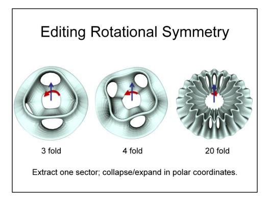
To edit rotational symmetry, we extract a sector of the model and collapse or expand that sector in polar coordinates. We instance the sector to complete the shape.
