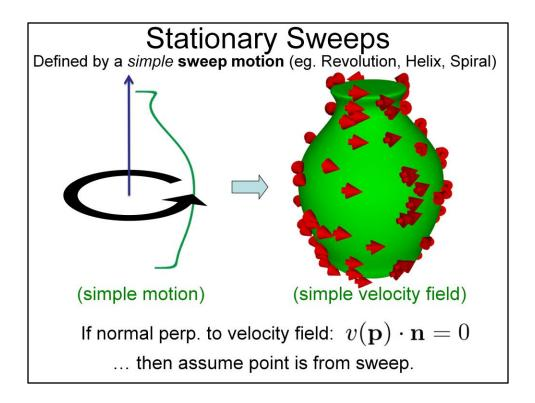
Our sweep module handles what we call stationary sweeps – sweeps defined by a simple sweep motion, such as surfaces of revolution, helices or spirals. These simple sweep motions correspond to following a simple, linear, velocity field – which enables a fast fitting algorithm specialized to these sweeps.
