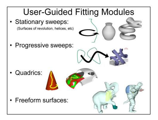
We currently have four fitting modules for different types of primitives: Two modules for different types of sweeps, a module for quadric surfaces, and a general freeform surfaces module.
