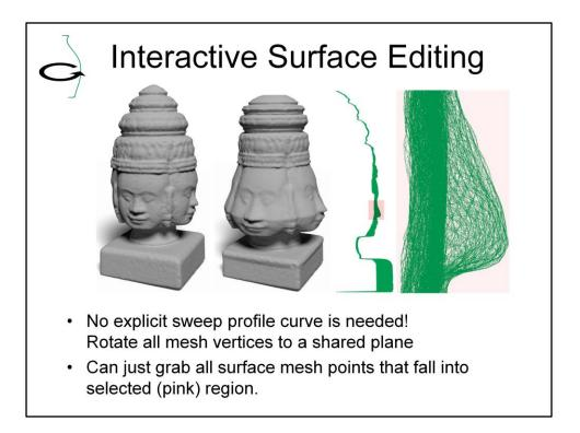
It's important to realize that we have just extracted all the surface elements that fit a particular equation, and we have not extracted an explicit profile curve for the sweep. However, "undoing" the sweep by rotating all mesh vertices into a shared profile plane can collapse the mesh into a "fuzzy" 2D cross section.
