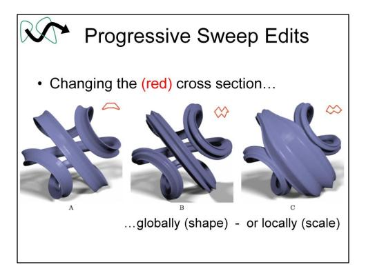
Once a progressive sweep has been fit, for example to the model on the left, we can start re-designing the extracted shape: for example by changing the shape of the cross section (shown in middle), or by changing one of the sweep parameters, such as the scale in some portion of the sweep (shown on right).
