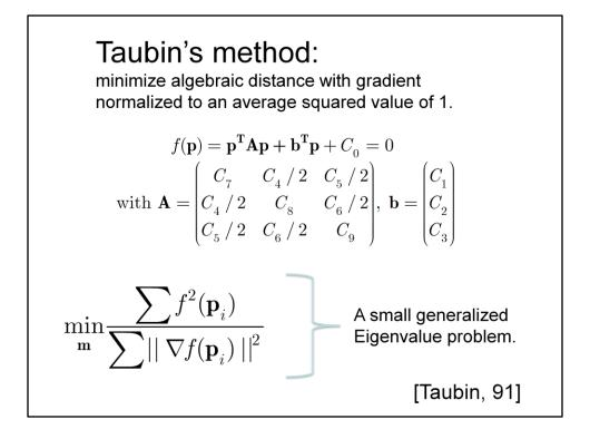
Taubin's method, like the stationary sweep fitting method, just requires the solution to a small generalized eigenvalue problem. This makes it very fast and easy to implement, and therefore appealing for an interactive system like ours.
