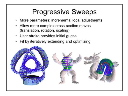
Progressive sweeps are a more general sweep primitive, good for any tubular shapes. For these primitives we actually extract an explicit cross section, and we allow that cross section to move along an arbitrarily complex smooth curve, while being smoothly scaled and slowly rotated.
