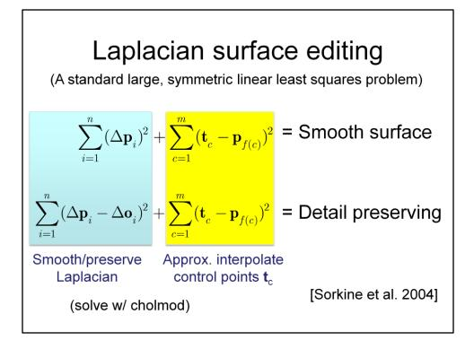
Laplacian surface editing is a smooth surface editing method that applies to arbitrary triangle meshes. By solving a large, sparse symmetric system, it can preserve or smooth surface detail by preserving or minimizing the Laplacians (left half of the equations, blue), while approximately interpolating constraints on the surface – points which the user moves manually (right half of the equations, yellow). We solve this linear least squares problem with "Cholmod": a direct sparse Cholesky solver.
