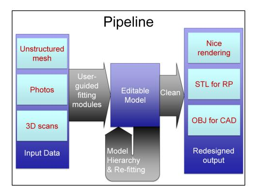
Our system will take low level input data, such a unstructured polygonal meshes or photographs, and through a user-guided fitting process generate an editable, parametric model that permits redesign. We let the users interactively re-fit shapes or impose hierarchical fits as needed. Once a satisfying redesign is created, we output a clean representation of the artifact for rendering, rapid prototyping, or further processing in a CAD system.
