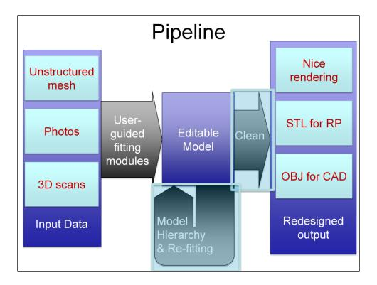
I've described our set of user guided fitting modules, and now move on to the remaining stages of our process: How we clean the model for export, and how we allow the user to impose hierarchy and change easily between differently parameterized representations.
