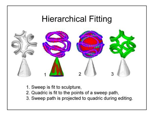
In addition to fitting primitives directly to the shape, our system also permits hierarchical fitting. For example, we fit a sweep to this sculpture, and then fit a sphere (red) to the points of the sweep path (magenta). We can then enforce the spherical structure of the sweep path by projecting points on the sweep path back to the quadric surface as they are edited.
