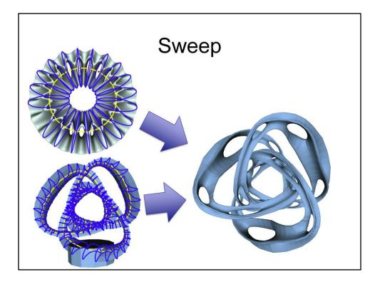
Again, even though the shape is not a sweep, the user can impose a sweep structure on the model and then reshape the model with a sweep-like editing operation, for example by twisting it into a trefoil knot as we do here.
