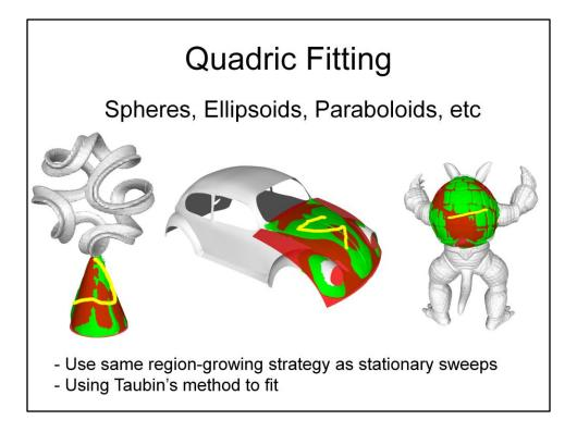
Our quadric fitting module functions similarly to our stationary sweep fitting module, starting from a user stroke and iteratively fitting and region-growing to extend the fit. To fit a quadric to a selection of points, we use Taubin's method (described next).
