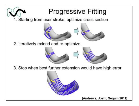
We initialize the fitting process with a sweep matching the model at the center of the user's stroke, and perpendicular to the stroke direction.
