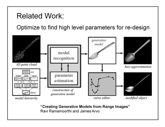
One inspiring work was a paper of Ramamoorthi and Arvo, which decomposed scanned models into parameteric representations which allowed some flexibility for later re-design.
