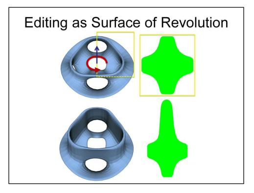
Even though this shape is clearly not a surface of revolution, the user can impose that structure on it. The vertices of the mesh are then rotated to a shared plane, creating the "cross sectional" shape shown on the right in green. By editing these vertices in that 2D space, and projecting the results back to 3D, we can for example extend the top flange of the model as we show here.
