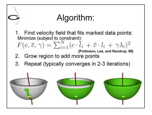
Our fitting algorithm starts from a user stroke on the model (shown in yellow). We then iteratively fit a sweep model to those points, and region grow to expand the selection to those surface points that also fit within some given error tolerance. The problem of fitting a field to any given selection is solved by a small (7x7) generalized eigenvalue problem, and the whole process tends to converge in only 2-3 iterations, making it very fast in practice.
