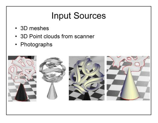
For this presentation, I'll focus on using 3D meshes as our source of input. We also plan to support input from point clouds and photographs. We have done preliminary work on supporting photographs: for example, from a collection of ten photographs of the sculpture on the left, we can extract the visual hull, (the 2<sup>nd</sup> image is an intersection of 10 silhouette cones). Then, with user hints, a sweep and cone are fit to the corresponding parts of the visual hull.
